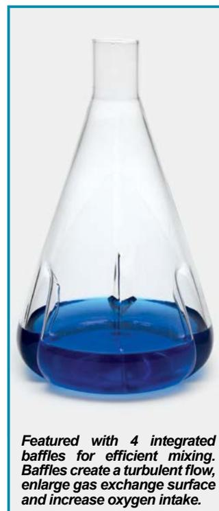
Featured with 4 integrated baffles for efficient mixing. Baffles create a turbulent flow, enlarge gas exchange surface and increase oxygen intake.
