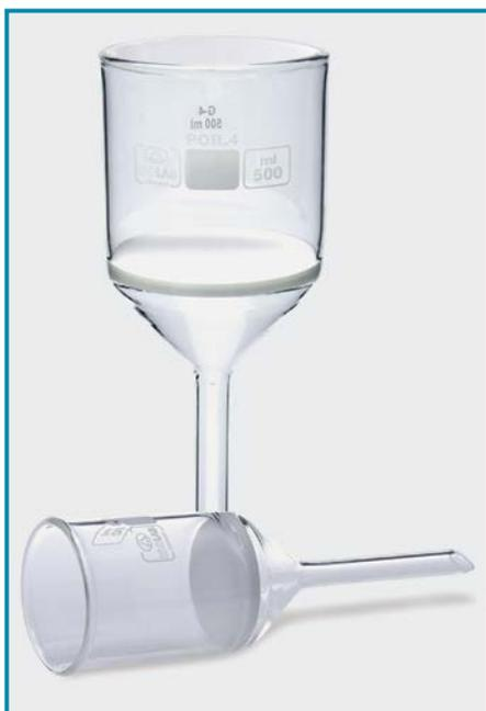
➤ Manufactured from heat resistant, durable borosilicate glass with an acid resistant sintered glass disc for filtration.
