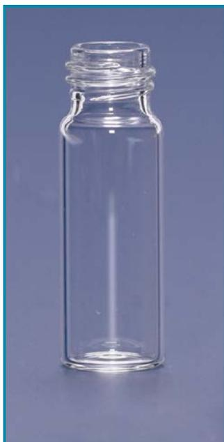
➤ Manufactured from hydrolic No:1 glass with perfect shape, very low dimensional tolerance and exact wall thickness for optimum performance.
