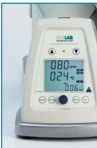
Integrated operating panel for convenient control of the main unit and also the heating bath.
