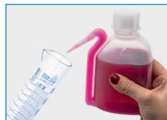
*Dispensing tip provides extra fine stream. The tip of the delivery tube can be cut in order to increase the liquid flow rate.*
