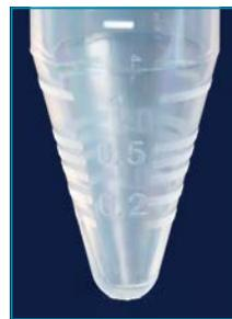
Precise volume marks at the tube bottom clearly and visually show the liquid volume at the tube bottom.
