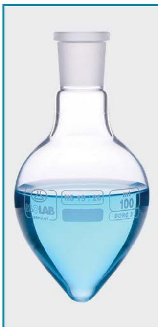
➤ Manufactured from heat resistant, durable borosilicate glass according to DIN 12383 standard.
